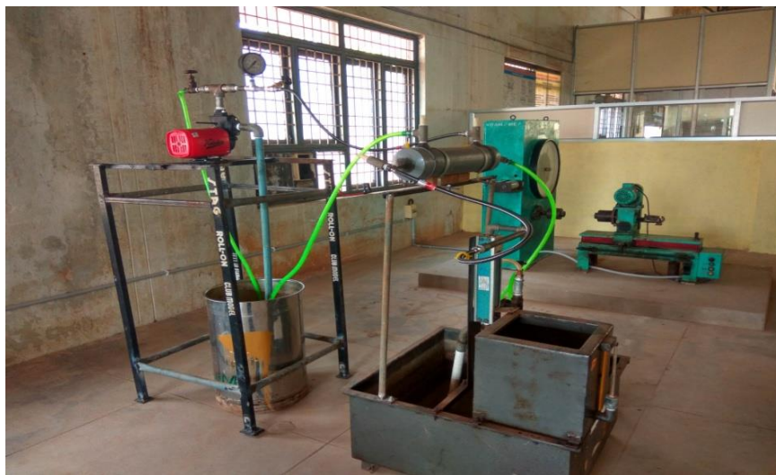
Fig. 1 Experimental setup of twisted helical tube heat exchanger
